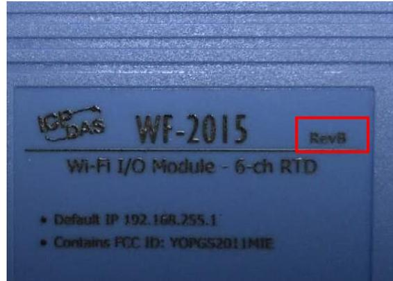
(b) Read the module settings via RS-232 and Utility. If the firmware version is B.x (x is the version number)
